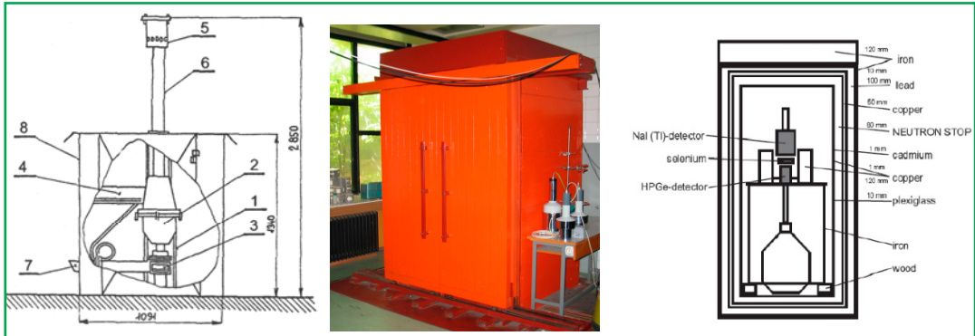
Figure 1 Scheme of the atmospheric aerosol-sampling device (left), and the low-level shield (right): 1 – construction, 2 – filter holder, 3 – pump, 4 – electronic regulator, 5 – separator of huge pieces, 6 – pipe, 7 – exhaust, 8 – shielding
