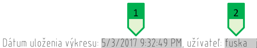
Fig. 88: Multiple fields inserted in one object of a single-line text, 1 – date field of the last saving of the drawing; 2 – name of the user who last saved the drawing
